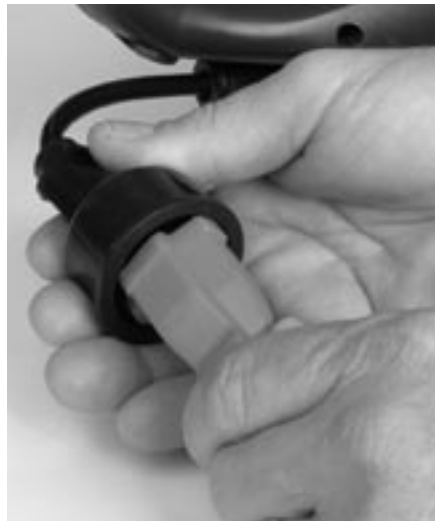
Figure 3-1: Plugging trimmer power cord into extension cord
